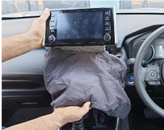
4 Remove 2x screws on side of digital display. Then, repeat for the other side.
