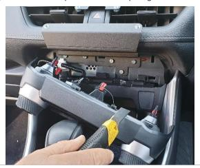
Replace the AC control back into its original location.
