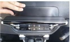
7 Loosen the AC module from the dash.
