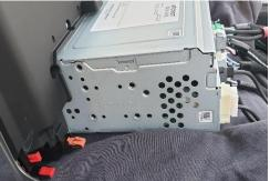
5 Fit supplied part underneath display and attach with the 4x screws removed in Step 4.
