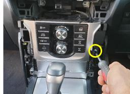
4 Remove 4x screws beneath digital display and lift display lightly. Do not remove / unplug.
