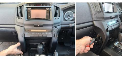
**5** Loosen and set aside left and right vents. Then, remove 2 x screws.
