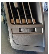
7 Install left and right brackets using previously removed screw. Then reinstall side vents.
