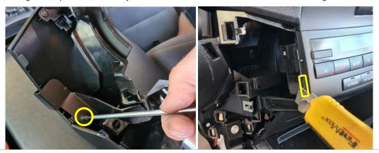
4 Reinstall side piece, side screw and panel to their original state.
