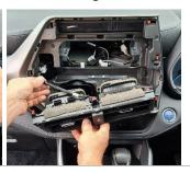
5 Place upper bracket into dash, using 2 x previously removed screws as a guide to secure 3 x self-tapper screws. The 2 x screws can then be removed.
