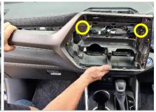
3 Install first bracket on removed dash component as indicated. Drill 2 x holes and secure to plate.
