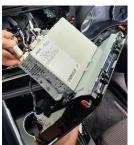
2 Loosen air vents, unplug, and set aside. Remove 2 x screws, then set aside dash component.
