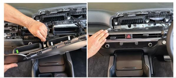
**11** Use 1 x previously removed screw to fix bracket in place as shown. Then use 1 x supplied self tapper screw to drill through the plastic and secure to the mounting point behind.
