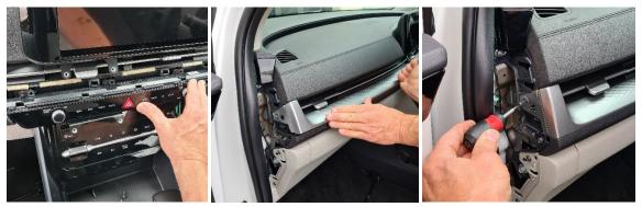
Install front dash bracket using 4 x provided screws.
