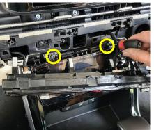
Install the second bracket using 2 x previously removed screws.
