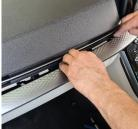
Remove 4 x screws. Then loosen indicated panel and remove 1 x screw.
