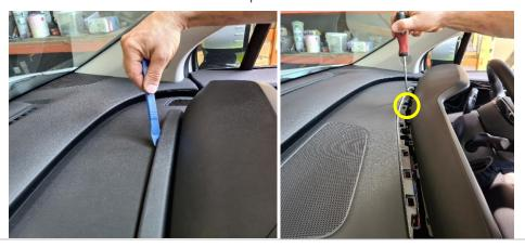
Loosen and remove plastic as indicated.
