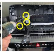
4 Lift forward plastic dash piece and install first bracket as indicated, fixing in place with 4 x screws.
