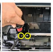
5 Trim internal tab off plastic dash piece as shown. Replace 1 x screw loosely, can't be too tight.
