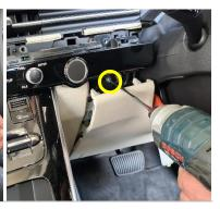
Loosen control panel, then remove 2 x screws.
