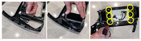
7 Using a sharp blade, carefully trim 2mm of plastic underside of the dash unit as indicated.
