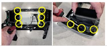
Install 2 x side brackets under the vents, then return 6 x screws
