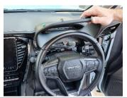
**2** Carefully loosen, then remove, the display unit. Plastic clips may break due to Isuzu design when removing front panel.
