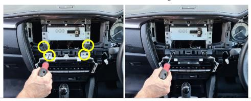
5 Remove 6 x screws on rear of display unit. Then remove 2 x vents, pressing down clips as shown.
