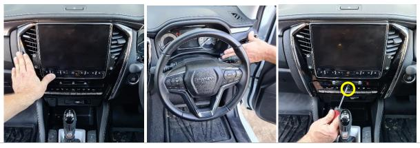
Install front dash bracket using 6 x provided screws.
