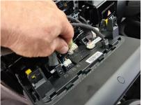
5 Remove screws as indicated. Then loosen indicated dash pieces, do not remove top panel.
