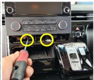
2 Loosen AC control unit, remove cable and set aside. Then remove 2 x screws.
