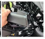
Remove rubber mat, insert plate, locate studs into holes, trim rubber mat re-install.
