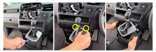
Remove 1 x screw, then loosen dash piece.
