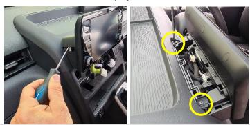
Loosen display unit, remove cables, and set aside.
