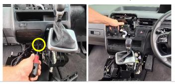
9 Move gearstick to neutral. Then unplug cables to remove dash component. Move the gearstick to park.
