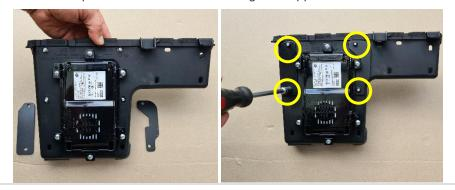
**13** Using a sharp blade remove 4 x tabs on the underside of the rubber mat and reinstall. Secure the hollow container back to the dash component using previously removed screws.
