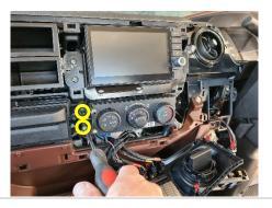
6 Using a sharp blade, carefully shave the indicated plastic extrusion from the internal dash piece.
