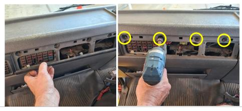
2 Loosen dash top and set aside, remove 2 x screws then install large bracket in place as shown.
