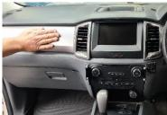
Fix front bracket into place using 4 x screw provided.
