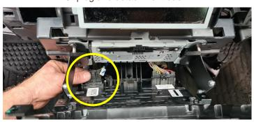
**8** Remove 2 x screw as indicated. Install right side bracket using original 2 x screws.
