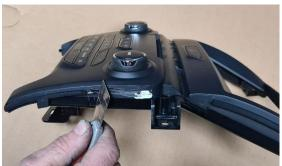
Plug 4 wires, press front console and fix into place using original screws previously removed.
