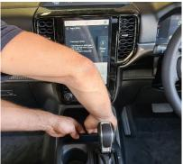
Then loosen and angle the gear stick surround as shown.
