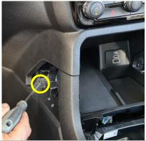
3 Loosen and set aside the internal dash tray, then remove indicated plastic part and store away.
